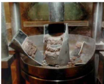
Breakout of the crucible following an electrorefining run
